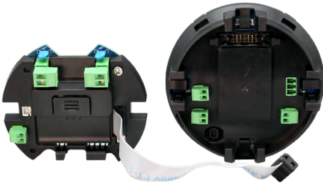
Options Board (Left) and Display Module (Right)
