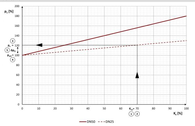
$p_1$ : Inlet Pressure  $K_{vx}$ : Flow coefficient at operating point  $p_{set}$ : set pressure of the valve  $p_2$ : Outlet Pressure  $K_{vs}$ : max. flow coefficient of the valve  $\Delta p_0$ : Opening pressure difference
