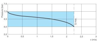
The plots are showing the reduced pressure falloff that occurs through the valve when the flow increases. Ensure that the operating conditions fall on the area depicted in blue for the recommended fluid flow velocity through the valve.
