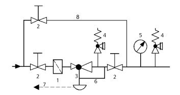
Sense line connection 10 - 20 x DN behind the valve
