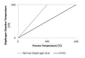
The HTDS is extensively tested in different circumstances and with various process temperatures. The graph presents the temperature reduction measured in the diaphragm chamber compared to a normal Diaphragm Seal. The HTDS is suitable for both gauge and differential pressure transmitters.
