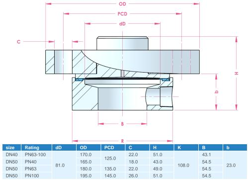
b size is based on lower part without flush
